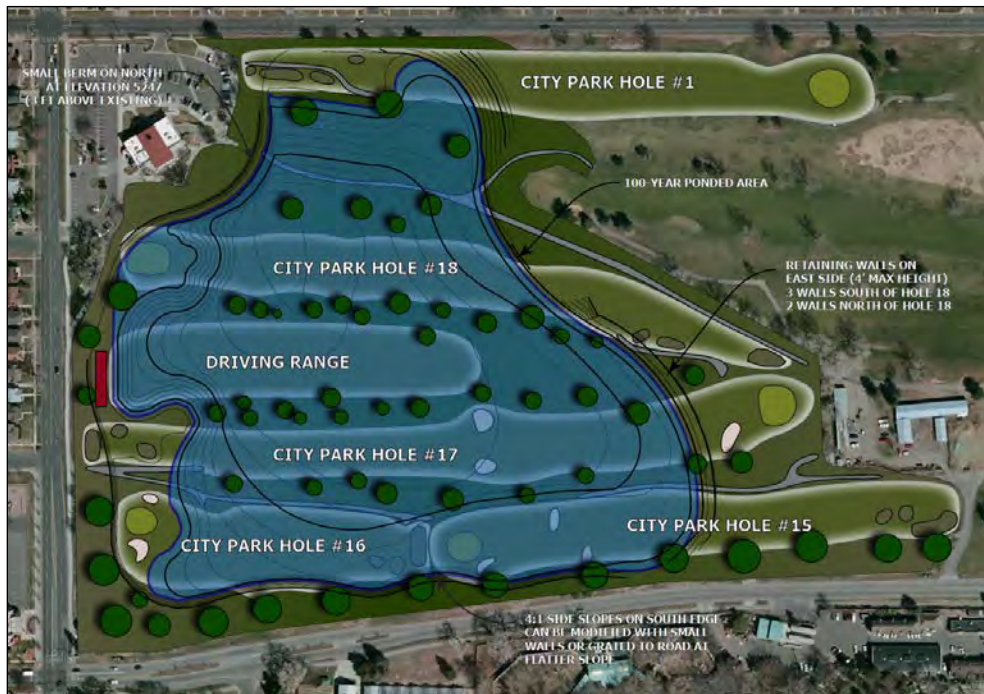
Figure 32. Concept Grading Plan Used for Feasibility Analysis
