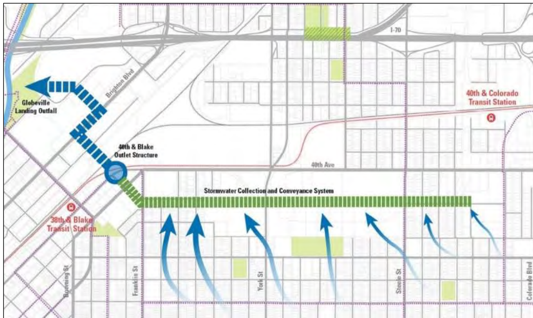
Figure 7. Montclair Basin Drainage Concept
